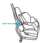
8. Remove remaining slack from the belt. Force the seat down with extra weight, e.g., by pressing down or kneeling on the child restraint while pulling up on the shoulder belt in order to force slack from the belt. This is necessary to remove the remaining slack that will exist once the additional weight of the child is added to the child restraint. It also helps to achieve the proper
